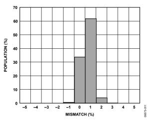
Figure 11. Self-Test Mismatch at  $25^{\circ}$ C ( $V_{RATIO} = 5 V$ )
