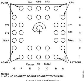
Figure 3. Pin Configuration
