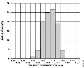
Figure 12. Current Consumption at 25°C ( $V_{RATIO} = 5 V$ )
