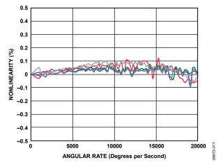
Figure 17. Typical Nonlinearity (Four Typical Devices)
