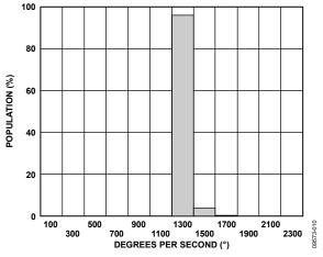
Figure 10. ST2 Output Change at 25°C ( $V_{RATIO} = 5 V$ )
