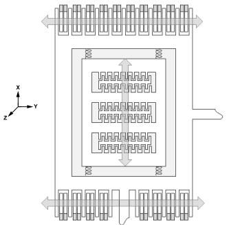
Figure 18. Simplified Gyro Sensing Structure—One Corner
