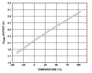
Figure 14.  $V_{TEMP}$  Output over Temperature, 256 Parts ( $V_{RATIO} = 5 V$ )
