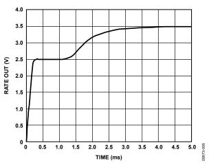
Figure 5. Typical Start-Up Behavior at RATEOUT
